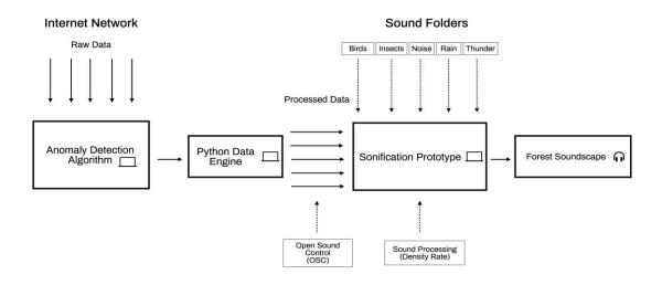
Scheme of the full system, designed by i3B-Ibermática and Sara Lenzi for Datascapes, from the collection of data from the digital network to its transformation into sound.
